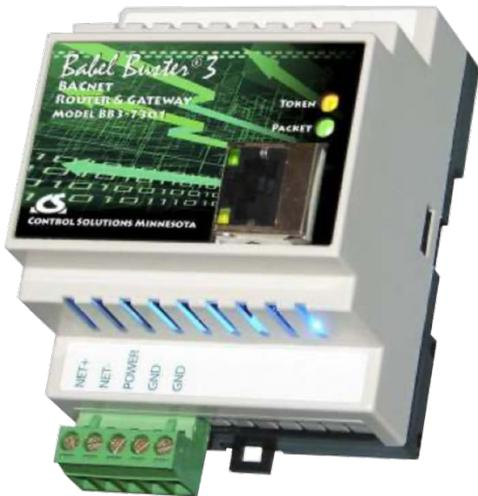
The IAQEye™ is designed to be easily integrated into an existing BACnet control system using a WiFi gateway called the Babel Buster® that translates the UDP measurement data relayed via WiFi from the transmitter into BACnet® objects used by a control system. Up to 200 IAQEye™ units can be used with one Babel Buster® (BB3-7302).
